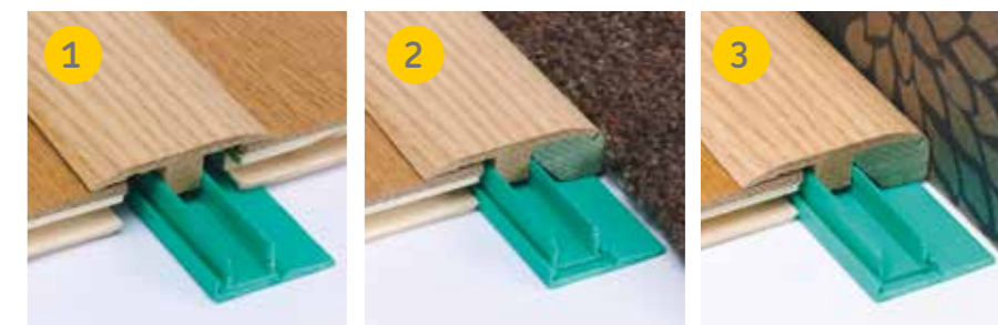
Expansion Profile to cover expansion gaps between two adjacent flooring products of the same height. Adaptor Profile for use when finishing between two adjoining floor coverings where the adjacent floor covering is of a lower height e.g. carpets or vinyl. Edge Profile to finish the flooring where a dressed edge is required eg. against a wall or window.
