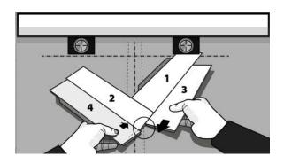
Make sure that the joint is closed tightly. Use hammer and tapping block to gently tap and ensure the locking mechanism is correctly engaged.
