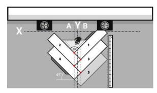
Having placed multiple planks in the centre row. Fill the open triangle close to the wall. Use the spacers to maintain the correct expansion gap between the wall and the floor. It is recommended to place some unopened boxes (or other type of weight) to keep the already installed section in place.
