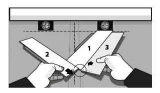
Now repeat the same method with plank (3) and (4). Plank (4) now serves as a stopper for plank (3). Fold down plank (3). Continue this process until you finish the center rows.
